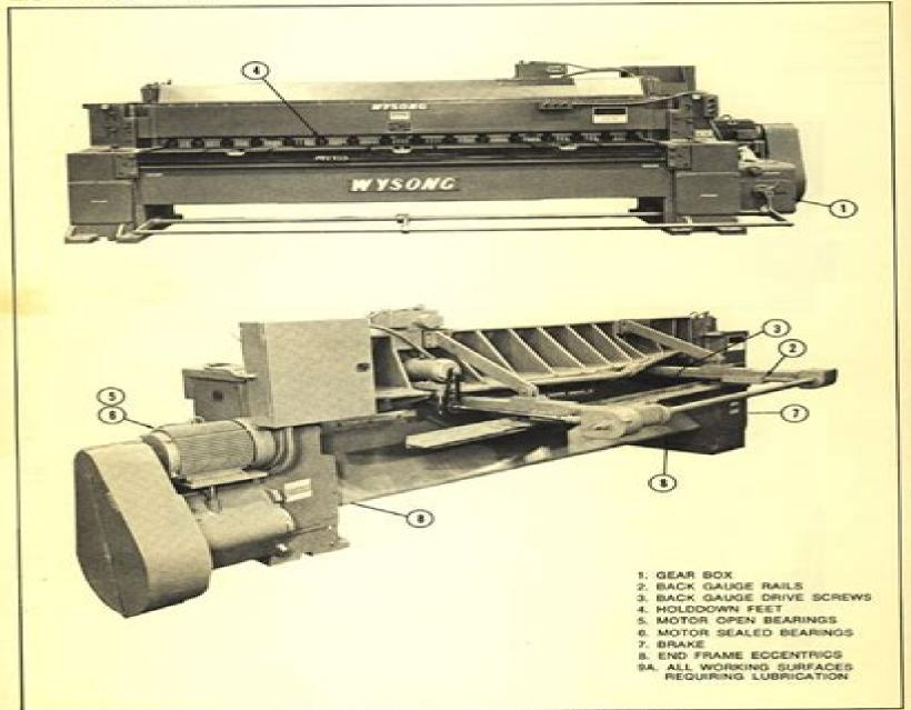
Fig. 18 - Lubrication - Double End Frame Shear.
