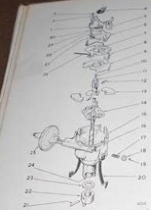
FIG 2:1 Distributor detains
