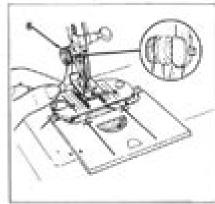
Bring thread from needle, under presser foot and wind it one turn in any direction, around presser foot sorine (8) pulling it into groove as shown.
