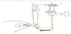
E. Squeeze needle threader grip with thumb and forefinger of left hand. Guide needle threader to the left, then raise it all the way up into the machine.
