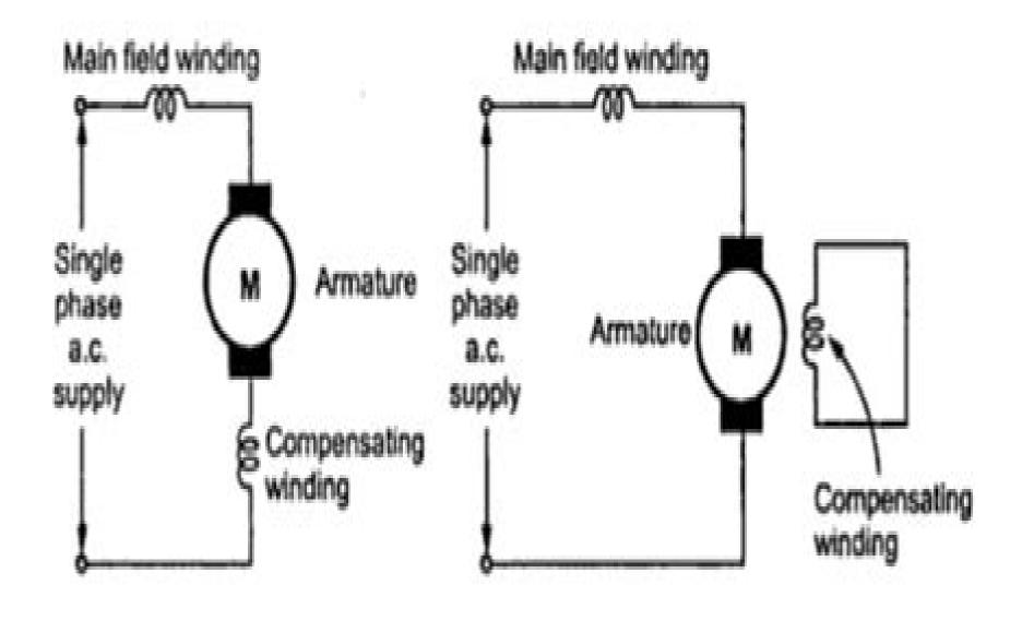
Conductively compensated motor
