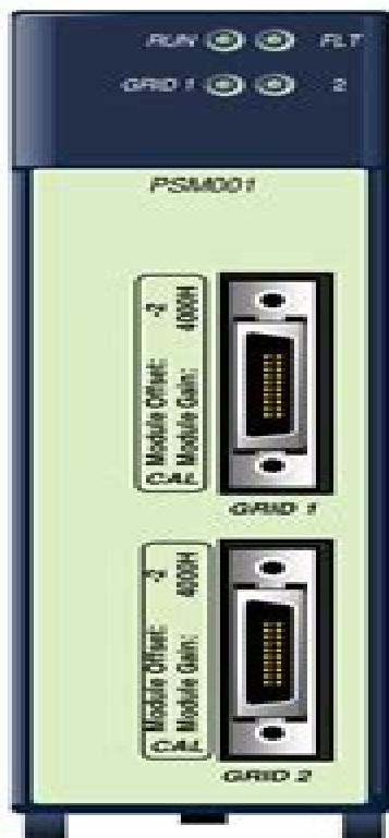
The PACSystems Power Sync and Measurement (PSM) system monitors two independent three-phase power grids. It incorporates advanced digital signal processor (DSP) technology to continuously process three voltage inputs and four current inputs for each grid. Measurements include RMS voltages, RMS currents, RMS power, frequency, and phase relationship between the phase voltages of both grids.
