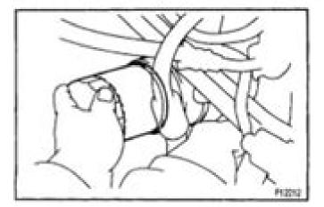
(d) Lightly screw the oil filter into place, and tighten it until the gasket contacts the seat.
